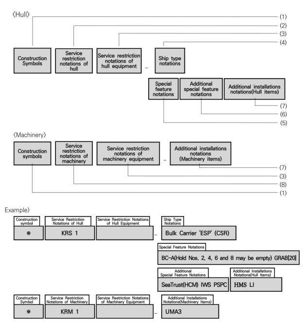
The Construction Symbols assigned to the ships according to the distinction of Classification Survey are to be in accordance with the followings:
